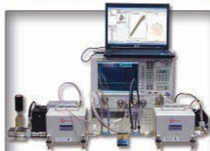
Pulsed-Bias Pulsed-RF Harmonic Load Pull for GaN and Wide Band-Gap Devices
