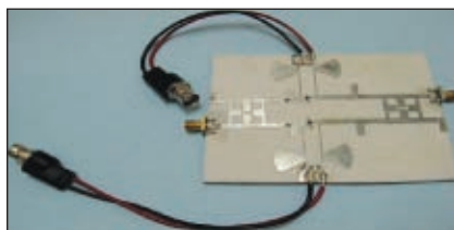
▲ Fig. 13 Photograph of the fabricated LNA.
