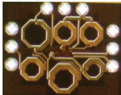
▲ Fig. 4 Photograph of the LNA with the modified shunt-peaking load.
